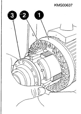
ASSEMBLING DEEP-GROOVE BALL BEARING ON INTERMEDIATE BEARING
